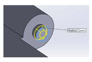
Sketch a concentric circle diameter 4mm on the hinge cut out, as shown.
