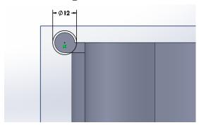
**Extrude Cut** this sketch **Mid Plane** at a distance of **45mm**.
