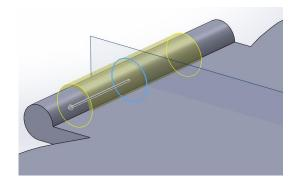
Sketch a concentric circle diameter **4mm** on the inner surface of the hinge
