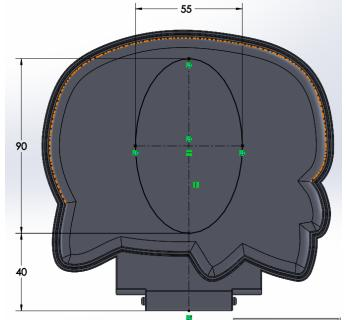
Extrude the ellipse 3mm with a Draft of  $45^{\circ}$ .
