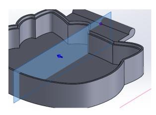
Insert a Plane using the Right Plane as first reference and the **midpoint** on the hinge the second reference.
