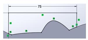
Extrude the sketch **Mid Plane** to a thickness of **10mm**.
