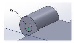
Extrude Cut to a depth of 3 mm.
