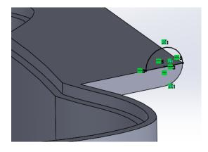
Create the semi-circular sketch on the side of the hinge.
