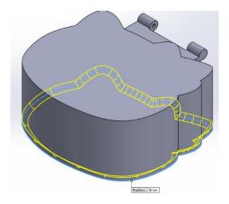
Shell the box to a thickness of 4mm.
